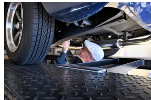
Brian Nass actively wrenching. Take differential out. Install new differential. Take out new differential with the long pinion flange. Re-install old differential. A lot of wrenching. Photo by A.J. Dowden
