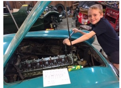
William torquing down the BN7 head
