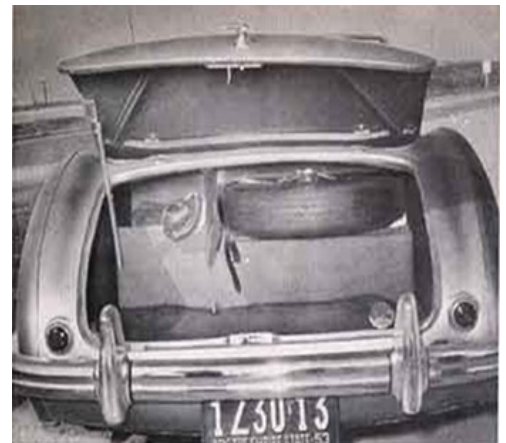
Despite the compactness of the Healey, the rear compartment affords plenty of room for luggage and spare tire. A master switch in the trunk cuts off all power.
