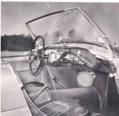
The drive shaft of the ground-hugging Austin-Healey divides the roomy seats.
