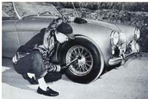
The wire wheels of Torme's special job are chromed but the production models come with painted wire wheels. Mel's car also has an all-aluminum body but the regular Austin-Healey "100", with an eye to traffic hazards, has steel fenders.
