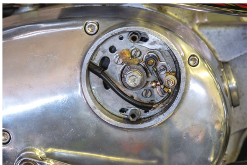
It's running! Check the timing. Is it advanced or retarded? And by how much? No marks!
