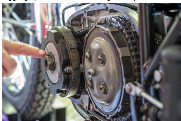
The B46's primary drive. Pointing to the crankshaft timing marks on the alternator cover. One is correct, the other
