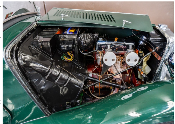
1947 MG TC engine. 1250cc, 54.5hp at 5200rpm. At 7.4:1 static compression and mild cam, the engine had lots of room for higher power modifications. Many were raced.
