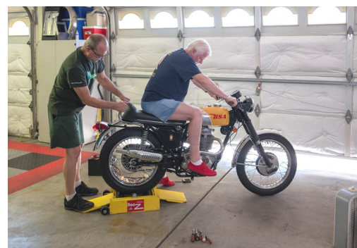
Trying to start the bike. Two starter motors drive rollers to turn the rear wheel while in second gear. This device is mostly used for starting high-compression race bikes. Starting a 441cc single cylinder engine with bad timing is more frustration and muscle aches than success. Good move, Bill.
