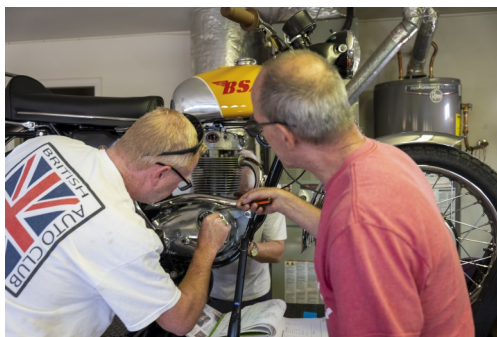
Jonas Payne and Gary Martin setting the ignition points timing. No timing marks! Set ignition timing, then try to start the engine. No start? Change setting. Once running, you can use a timing light.
